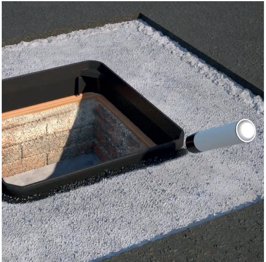
A typical example of cold joint sealer application is shown in illustration.
